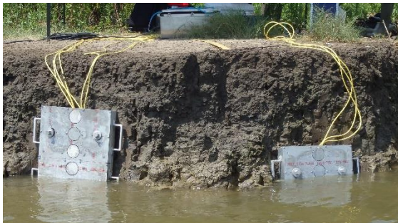
Figure 1 – Photo of two load cell arrays measuring vessel wake forces on a marsh scarp in Louisiana, USA
