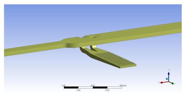
Figure 14: Culvert Connection to Bottom Grid
