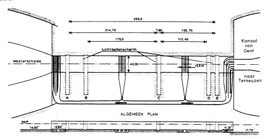
Figure 2: General Plan West Lock: Two Bottom Grids Centered Between Inner Gates
