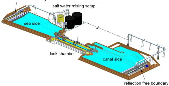
Figure 6: Scale Model Design IJmuiden Lock and Terneuzen Lock
