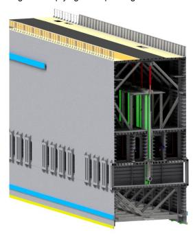
Figure 9: Cross-section Rolling Gate
