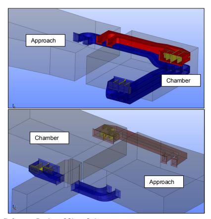
Figure 8: Reference Design of Short Culverts
