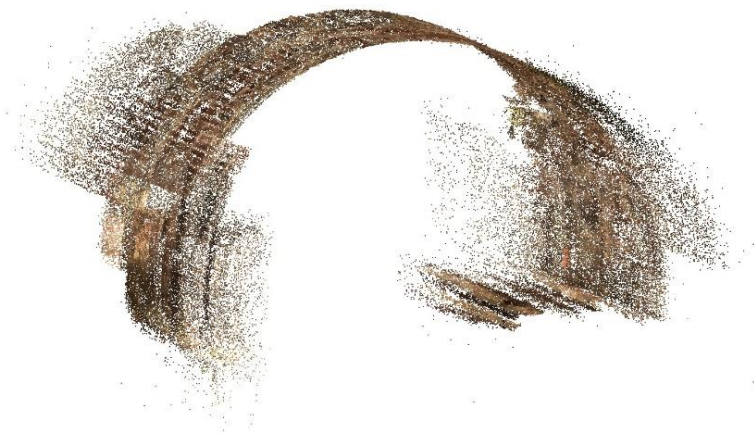
Figure 13: Tile registration using Photoscan® software
