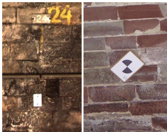
Figure 10: Examples of targets viewed in the images. Catadioptric plate (left) and lasergrammetric target (right)
