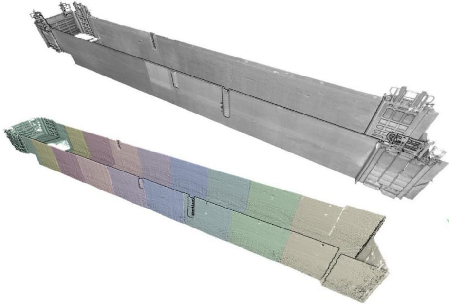
Figure 4: Complete model of the lock from terrestrial laser scanning (top) and mechanical sonar scanning (bottom). Colours represent the scans of the 9 sonar static acquisitions
