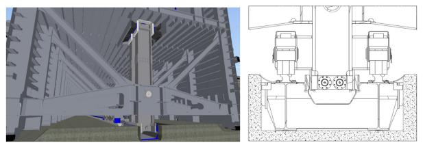
Figure 10: Cross section of horizontal guidance structure and rail beam structure
