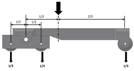
Figure 17: Load distribution upper carriage
