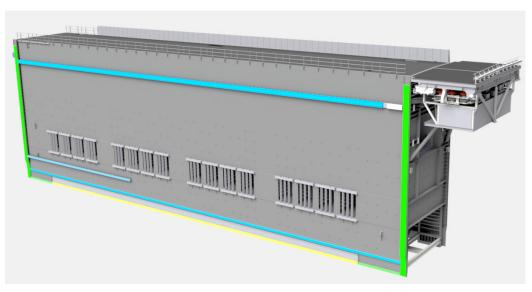
Figure 2: New rolling gate (72x25x11 meters)
