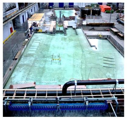
Figure 12: Scale (1:40) model test
