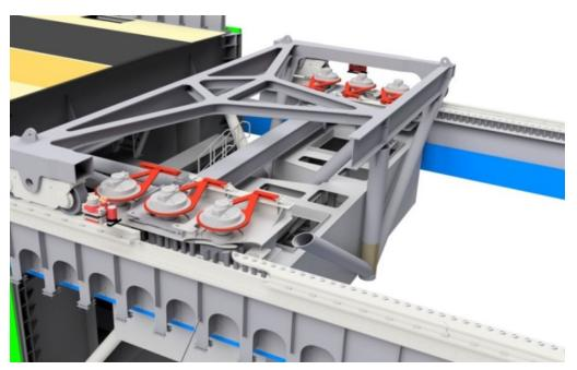
Figure 18: Pinion - pin track drive
