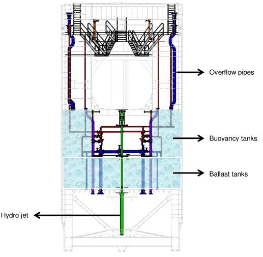
Figure 8: Filling and emptying system of the buoyancy tanks
