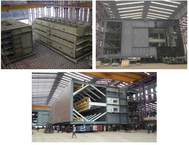
Figure 20: Steelwork fabrication of the lock gates in South Korea
