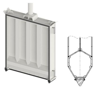
Figure 13: Sluice gate and cross section of bottom girder
