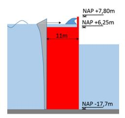
Figure 4: High water retaining function
