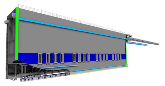
Figure 6: Wheelbarrow type rolling gate with horizontal sliding pads
