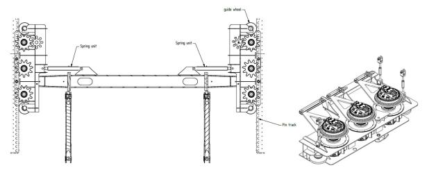
Figure 19: Suspension of drive trains
