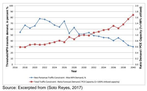
Figure 2. Expanded Panama Canal capacity, 1-run dynamic forecasting
