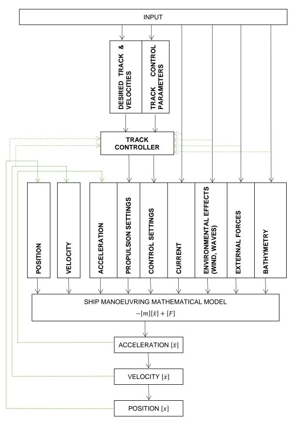
Figure 5 Calculation scheme of Fast-time Track Controller
