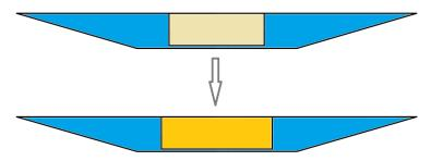
Figure 7 Smallest theoretic cross section of the Canal Ghent Terneuzen with midship sections of a ship BxT 37x12.5m<sup>2</sup> and 43x12.5m<sup>2</sup>
