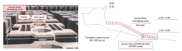
Figure 19 : Armour blocks attached with EAC panels and Cross-section
