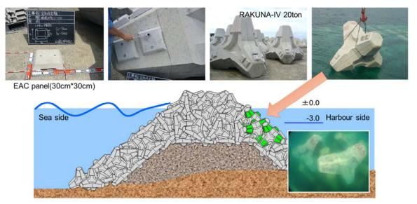
Figure 15 : Wave-dissipating block attached with EAC panel and Cross-section
