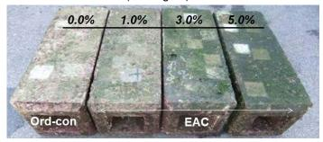
Figure 11 : Monitoring condition of blocks taken from underwater after 8 months
