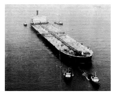
Figure 2: The 318t deadweight oil tanker SS Lepton was a subject of investigation for the full scale experiment at the Port of Rotterdam in 1974. Here, SS Lepton is filled with water enters the Port of Rotterdam. Observers on board carefully follow the sailing behavior of the ship. The Lepton was 350 m long and 55 m wide, the draft was 20.90 m, the average throat clearance was 1.60 m, the average mud layer was about 1.15 m. The photo is taken from Nederlof, L. (1979).
