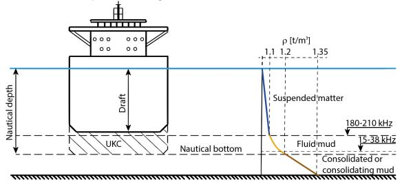
Figure 1: The nautical bottom concept, which was developed at the density limit of 1.2 t/m<sup>3</sup>. Adapted from from Nederlof, L. (1978).
