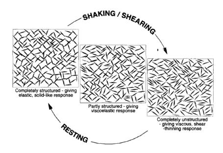
Figure 6: Breakdown of the thixotropic structure. Taken from Barnes, H. A. (1997).
