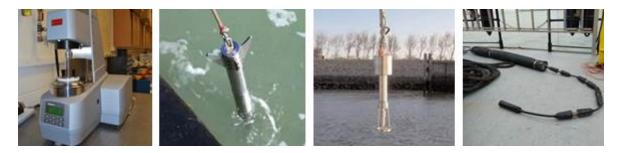
Figure 7: Examples of rheology-based methods. From left to right: lab rheometer (Anton Paar), free falling cone (Graviprobe), tunning fork (Rheotune), towing object (Rheocable)
