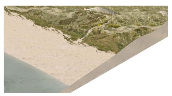
Figure 13. Cross section of the new western beach section with dunes at Lolland
