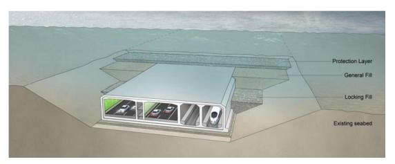
Figure 2. Cross section of dredged trench with tunnel element and backfilling
