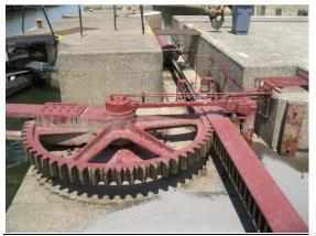
Fig. 5: Ohio River Linkage with rack gear and sector gear
