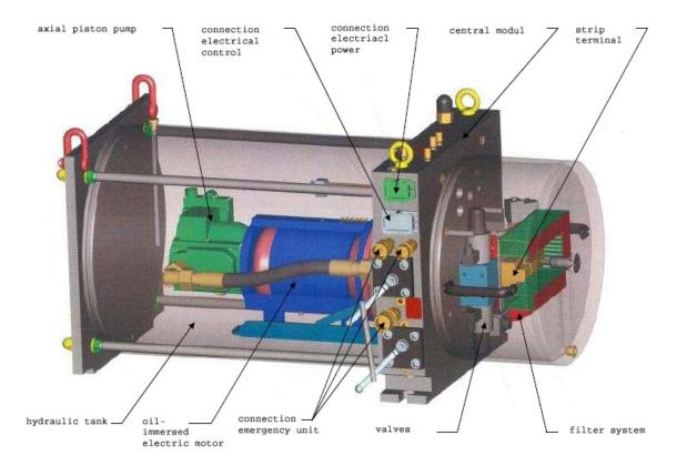
Fig. 10: Hydraulic Compact Drive unit - general arrangement
