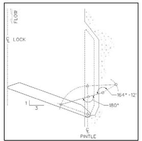
Fig. 3: Modified Ohio River Linkage
