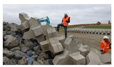
Figure 5 - Xbloc placed on a test slope
