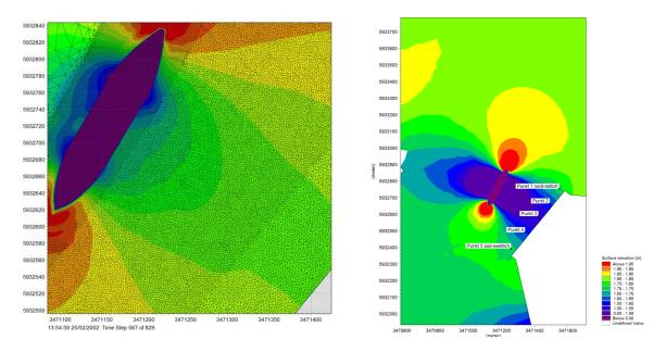
Figure 6: Passing ship hull included in the mesh and the calculated drawdown in front of the OTB
