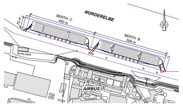
Figure 10: Extended mooring facilities in Finkenwerder, Hamburg
