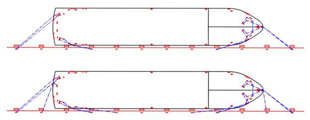
Figure 7: Mooring arrangements of the cargo ship P2-800. Upper panel: Initial mooring arrangement, Lower panel: Optimized set up with additional mooring lines.
