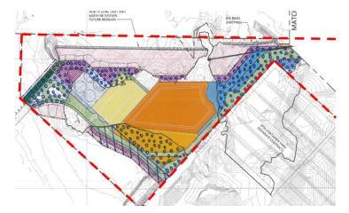
Figure 3: Cut and fill areas at project start date (access road is not shown) (fill shown with handmade hatch, red discontinued line is concession boundary, pink area is initial unsuitable fill material disposal area)
