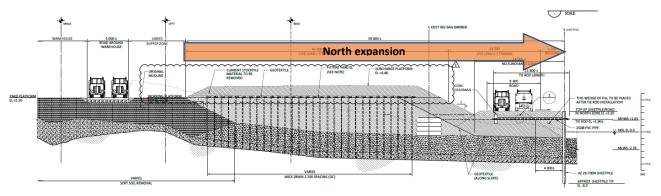
Figure 10: Cross section north yard with typical surcharge (here 1,5m high for 2t/m<sup>2</sup>)
