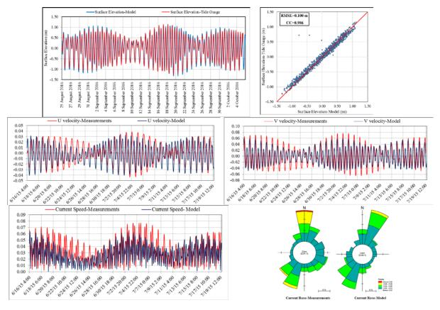
Figure 4: Comparison of predicted and observed surface elevation and tidal current speed at Roudic station
