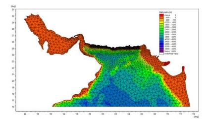
Figure 3: Hydrodynamic model mesh and bathymetry
