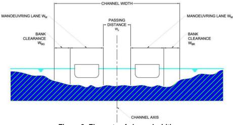
Figure 2: Elements of channel width
