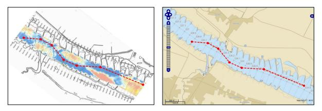
Figure 2: Construction of a recommended track, visualized in Inland ECDIS
