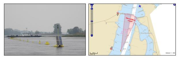
Figure 3: Cable ferry at the river Elbe, virtual caution area while the ferry is crossing
