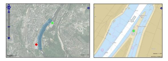
Figure 5: Current switching status of signals, visualized in Inland ECDIS
