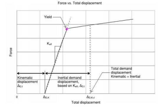
Figure 3: Pushover Curve for Kinematic plus Inertial Analysis
