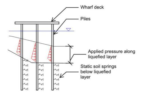
Figure 4: Kinematic Load Applied as Fluid Pressure
