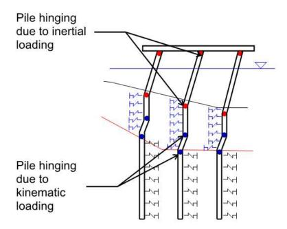
Figure 2c: Combined Pile Hinge Locations for Inertial and Kinematic Loading
