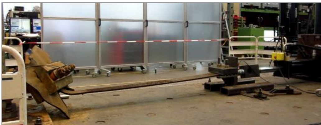
Figure 6: Testing of a rubber sheet in the clamping system
