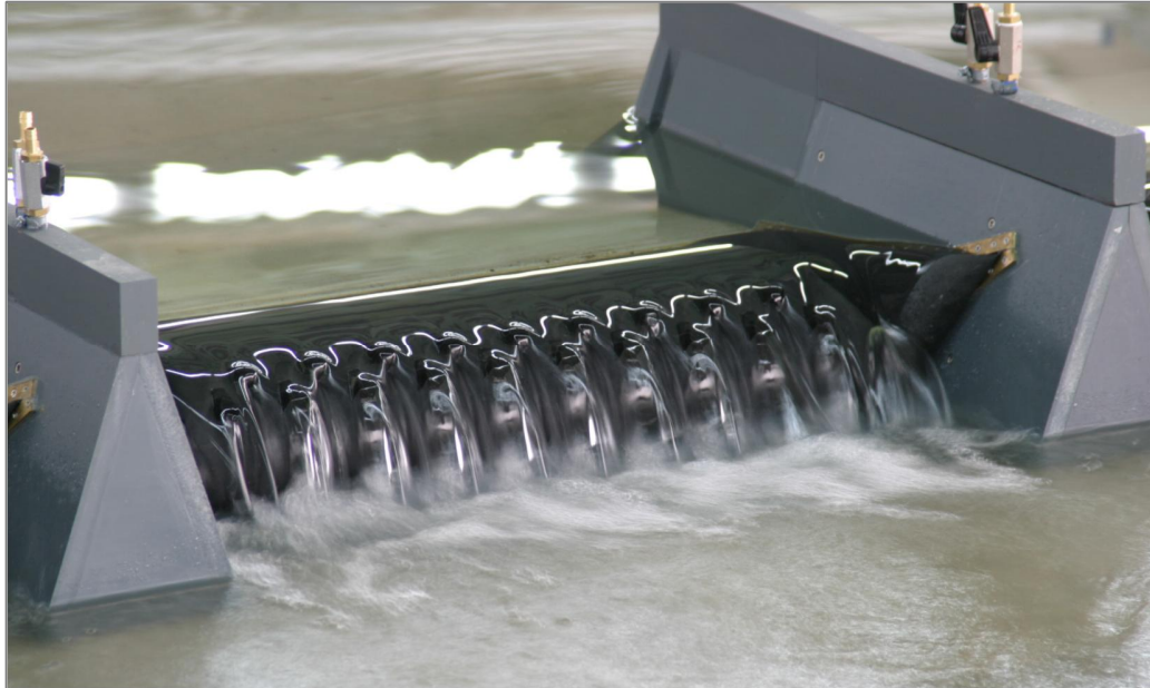
Figure 10: Scale model of a rubber gate with breakers
