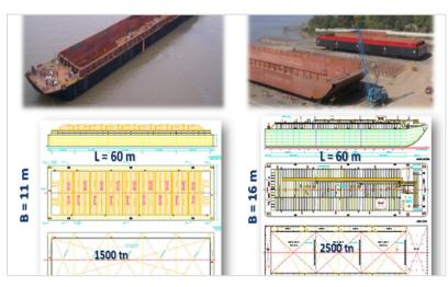
Figure 3 – Dimensions of "Mississippi" and "Jumbo" barges
