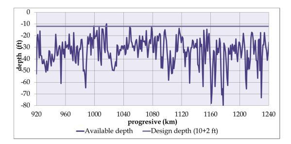
Figure 10 - Longitudinal profile of the river
