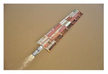
Figure 5: Example of a 6 x 7 barges convoy
