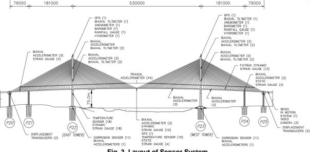
Fig. 3. Layout of Sensor System
