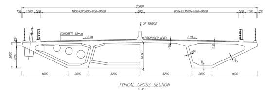
Figure 2: Typical section of deck
