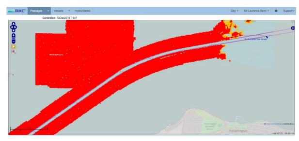
Figure 9 Geelong Chart Overlays: UKC critical locations are highlighted.
