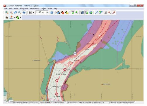
Figure 4 Chart Overlay (Source: Internal). Pilots have direct access to real time UKC information via the PPU.
