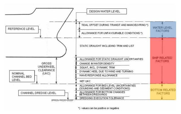
Figure 1 Channel Depth Factors (PIANC, 2014)
