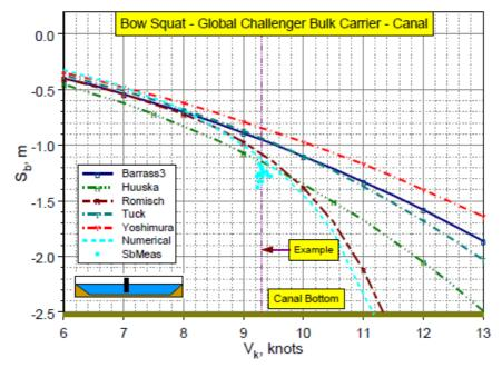
Figure D-13: Bow squat for Global Challenger Bulk Carrier, Panama Canal, L<sub>pp</sub> = 216 m, B = 32.2 m, T = 11.7 m, C<sub>B</sub> = 0.83, h = 14.2 m (h/T = 1.21), W = 152.4 m, W<sub>Top</sub> = 206.4 m and n = 1.9
