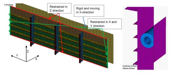
Figure 6: design hull section FE model, original case: no constraints in x-direction on web frames
