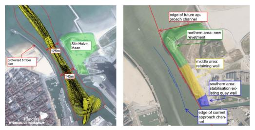
Figure 1: navigation simulation with widened approach channel and definition of project zones
